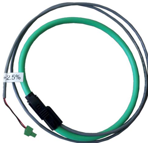
Self-powered rope CTs have a fixed amperage of 4800A. Each has slightly different output characteristics and because of that, each comes labeled with a calibration sticker. For accurate operation, the value printed on the calibration sticker has to be entered into the eGauge configuration. Specifically, to configure a *self-powered* rope CT, select "Rope 6" from the appropriate CT drop-down menu. For example, if we do this for CT1, then the entry area will look like this:
