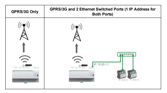
GPRS/3G access can be added to the Com'X 510 by installing a modern under the cover.
