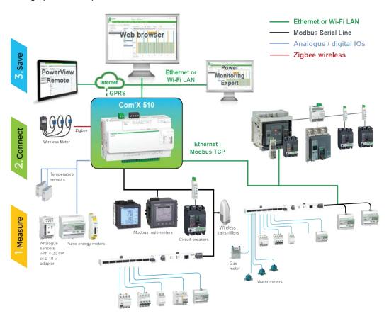
From a simple metering installation with one device to large metering systems, the Com'X 510 collects data from any Modbus TCP/Modbus serial line gateways, pulse meters, actuators, and analog sensors.
