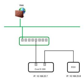
In switch mode, both Ethernet ports have the same settings. Using two ports simplifies wiring:
