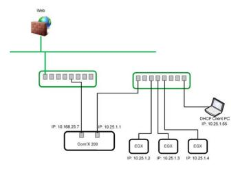
In upstream/downstream mode, the two Ethernet ports have different settings and function independently:
