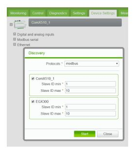
Follow this procedure to discover connected Modbus devices:
