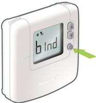
The symbols start flashing. If the Honeywell HGI80 communication module and the Smart thermostat DT-92 have connected successfully, the symbols stop flashing and remain visible on the screen of your Smart thermostat DT-92. The red led on the receiver fades out. Every time the Smart thermostat DT-92 communicates with the platform, the symbol flashes.
