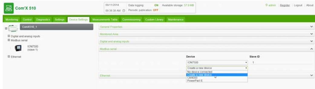
Follow this procedure to add a Modbus serial device (for example, PM710 meter):
