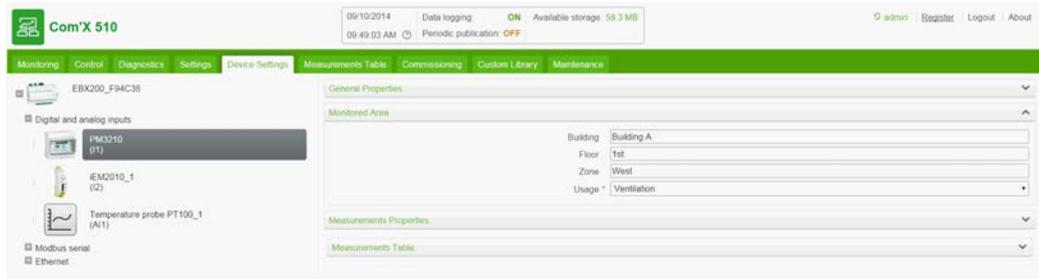
This area enables you to define the building area measured by the meter or sensor. A site can be made up of several buildings. Each building can have several floors. Each floor can be made up of several zones. The site topology is defined by entering values in the **Building**, **Floor**, and **Zone** fields.
