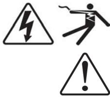
The addition of either symbol to a "Danger" or "Warning" safety label indicates that an electrical hazard exists which will result in personal injury if the instructions are not followed.
